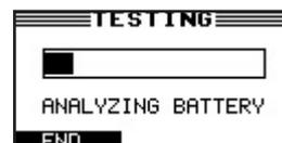
When the battery has a low state of charge the charger will ask you if you want to charge the battery first prior to starting the power supply function. It is advised to do this because ECU programming with a battery in a low state of charge can cause damage to the ECU when the battery voltage drops below a certain limit.
