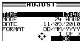
A scrolling list contains items that extend above and below the screen. The first number above the right soft key indicates the position in the list of the highlighted
