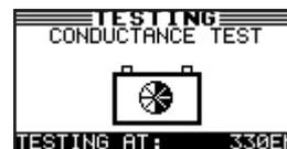
The next step is to apply an electrical load and test the response.
