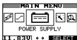
2. Use the **UP (▲)** or **DOWN (▼) ARROW** key to select the **BATTERY TYPE**, or press the corresponding numerical keys to move the dot to the option button of your choice.
