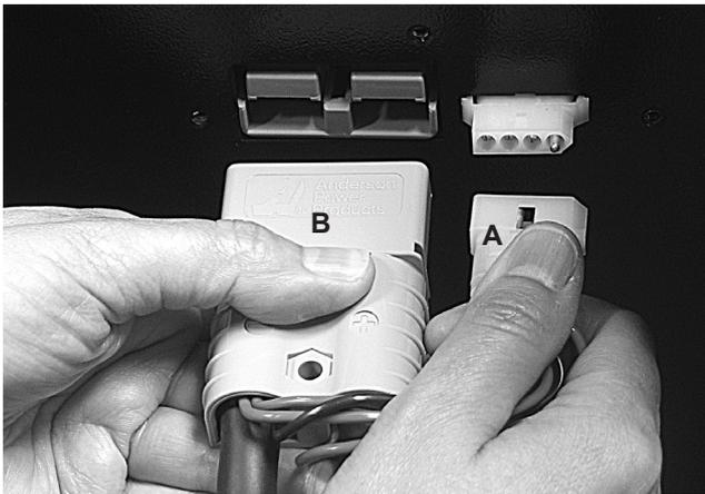
2. Plug the large connector (B) into the large socket while placing the protective cover (C) against the back of the unit.
