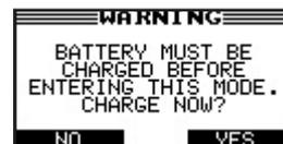
If **YES** is selected the battery will be charged in the Diagnostic Charge mode until it is ready. It will automatically jump back to the Power Supply screen and maintains the battery with the selected voltage threshold.
